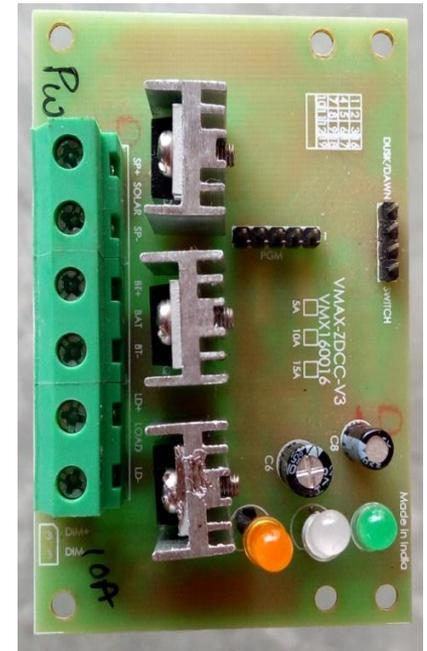
**PWM Solar charge controller 5A-20A**
