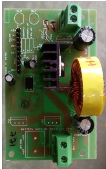
**Microcontrolled DC-DC LED Driver: 20W to 50W**
