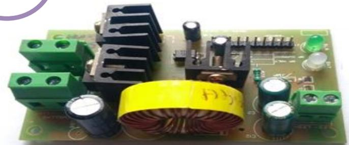
**Solar charge controller with LED driver (Combo driver): 6W to 50W**
